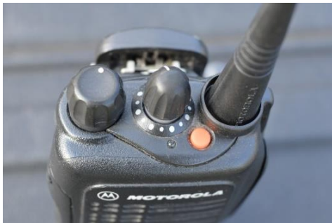
Controls GP-Class Motorola: Left: On/off and volume switch, center: Channel selector switch
