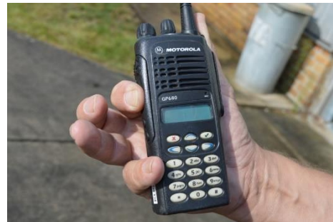
The PTT key is usually operated with the index or middle finger
