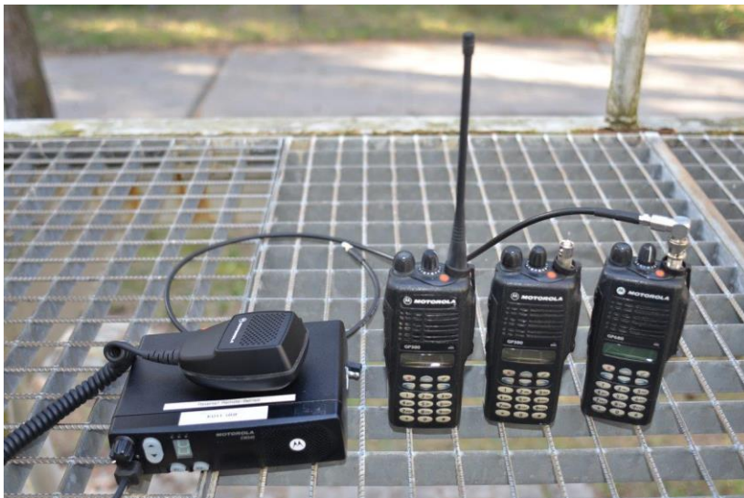
Typical wireless technology, from left to right: Mobile device CM 340 with handheld microphone for use in vehicles (12 V electrical system); Handheld radio GP 380 with flexible standard antenna; GP 380 with BNC-adapter and GP 380 with BNC-adapter / plug and coaxial cable for connection to a remote antenna
